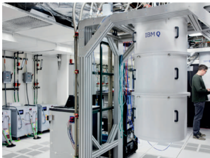
Figure 76: multiple IBM Q systems in the IBM Q computation center. – Source: IBM
