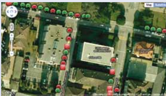
Parkomotivo: the parking monitoring wireless sensor network deployed in Lugano.
